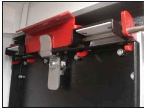
Cam, door and the Claw Locking Mechanism engaged on box.
