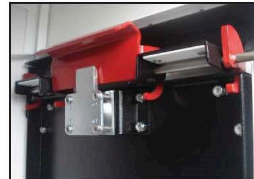
Deadbolt, door and the Claw Locking Mechanism engaged on box.
